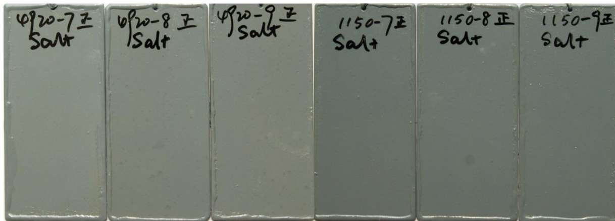
“EpoxyThane” in Salt Water -30 Days
