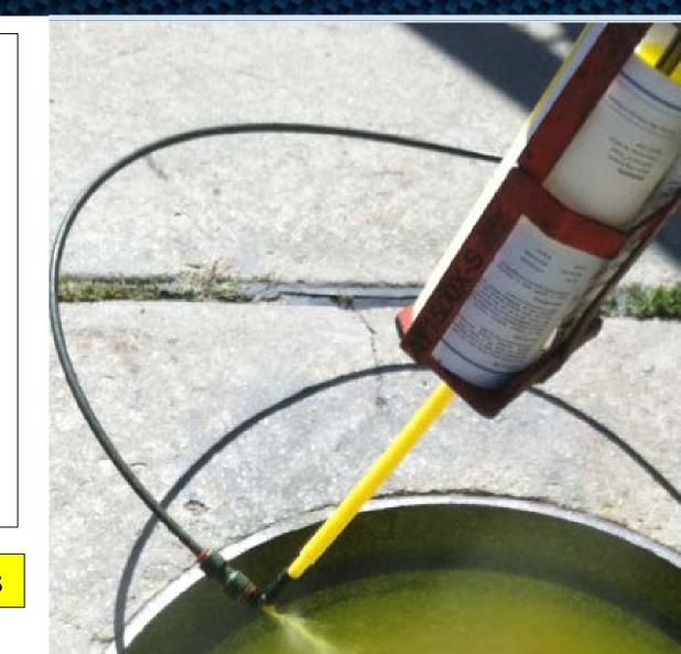
**Consistent Yellow Color = Proper film thickness**
